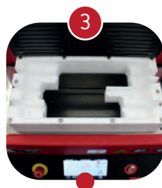
Bigger shrinking fixture comparing to standard STCS-VMir: 225mm x 100mm
