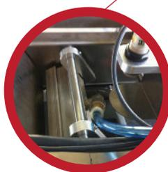
Optional cooling system, based on compressed air amplifiers, to cool down the splices after processing and prevent the cables from sticking
