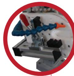
Can be supplied with customized clamps with automatic holding systems and/or cooling system
