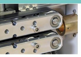
Prefeeders from Metzner are used when material is dereeled from a device without a drive. These include cable and profile reels, coils, loose rings or processing directly from a box or cable rack.
