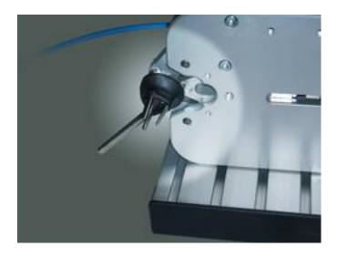
With this three-pronged device flexible grommets can be expanded. The cable or hose is easy to put through the widened opening.
