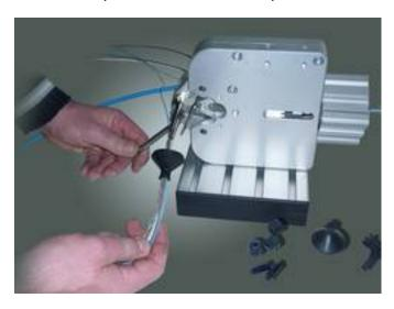
For better handling there is a hand lever on the tool. This makes removal of assembled harnesses easier.
