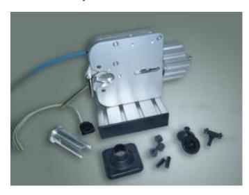
Commercial description for this type of tool: **EXPANSORA TRES**With an air pressure of 6 bar the pneumatic device is ready for operating.
