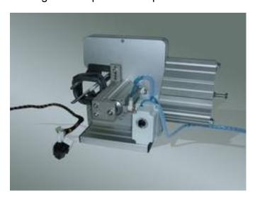
The grommet will be expanded carefully by activation of the tool. The speed and size of the widening is infinitely variable.
