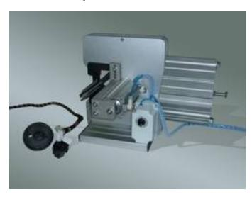
The tool **EXPANSORA QUATRO incl. Pull-off unit** is designed for large, heavy grommets. (Fire-wall-grommet, Car body grommet) In the standard size of the tool the degree of expansion is up to 100 x 100 mm. Larger expansions are possible.
