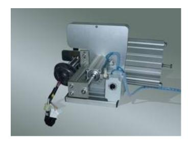
The grommet will be assembled reliably by activation of the Pull-Off Unit.
