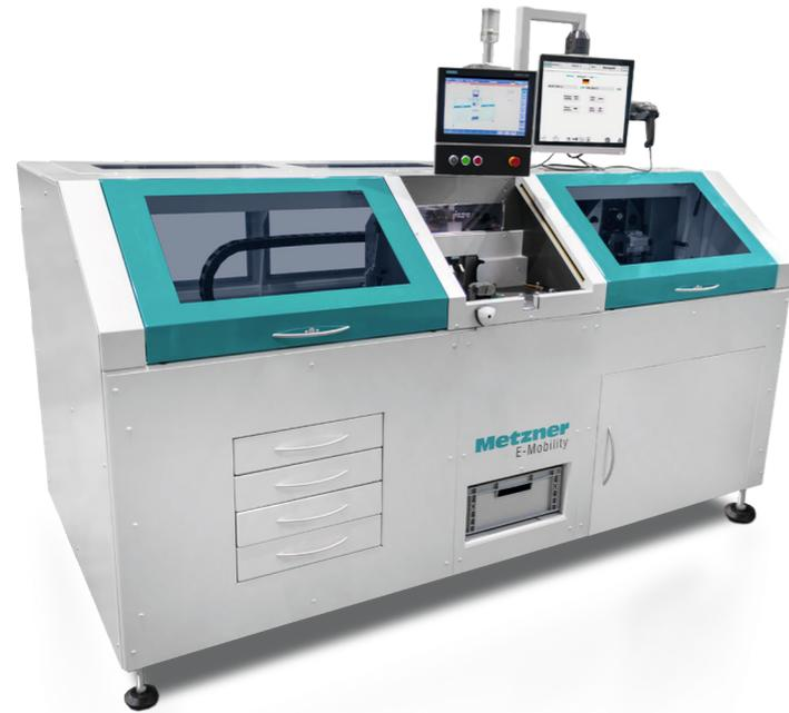
The EM 600 is able to combine up to 6 consecutive process tools in one station. After insertion, the cable remains in a fixed position while the tools move to the cable for optimal protection of the HV cables. The total cycle time of an EM 600 station is approx. 30 s for all processes of this station, with a total capacity of approx. 400,000 cable ends per year.
