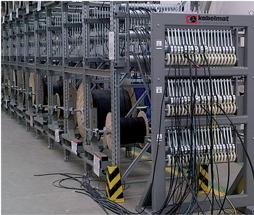
Fig. 1 TROMBULLY with central point of removal and return stop
