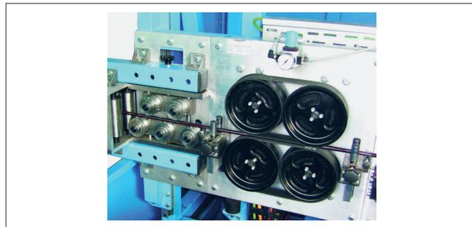
Fig. 2 MESSBOI BELT installed in a machine with roller cages and straightening element
