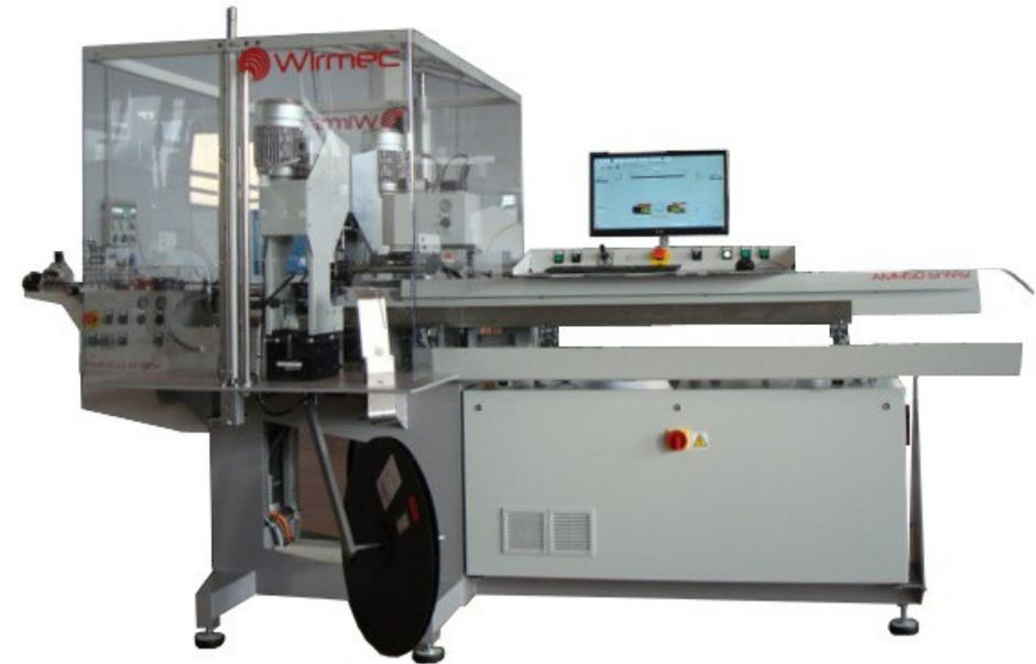
Cut strip and terminate machine derived from more bigger AM500, can be equipped up to five processing stations.
