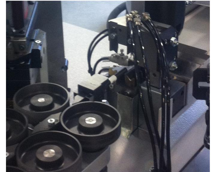
Feeder in the advanced position close to the cutting head, for the processing of very small section of cable. It can be powered that both roller belt
