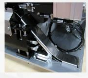
The machine is provided with currier strip guide for the applicators without cut currier strip.
