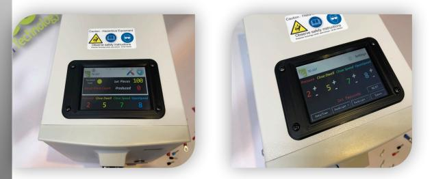
The all electric TC-15T terminal crimping machine is simple to operate and requires no compressed air. By the use of a foot switch activating the machine cycle, this leaves the user free to use both hands to accurately position the wire and terminal.
