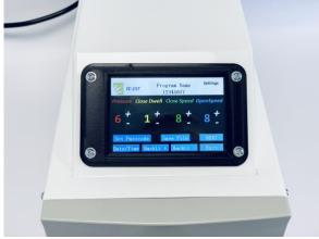
The all electric TC-15T terminal crimping machine is simple to operate and requires no compressed air. By the use of a foot switch activating the machine cycle, this leaves the user free to use both hands to accurately position the wire and terminal.
