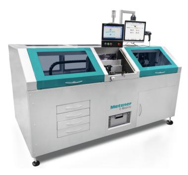
The EM 600 is able to combine up to 6 consecutive process tools in one station. After insertion, the cable remains in a fixed position while the tools move to the cable for optimal protection of the HV cables. The total cycle time of an EM 600 station is approx. 30 s for all processes of this station, with a total capacity of approx. 400,000 cable ends per year.
