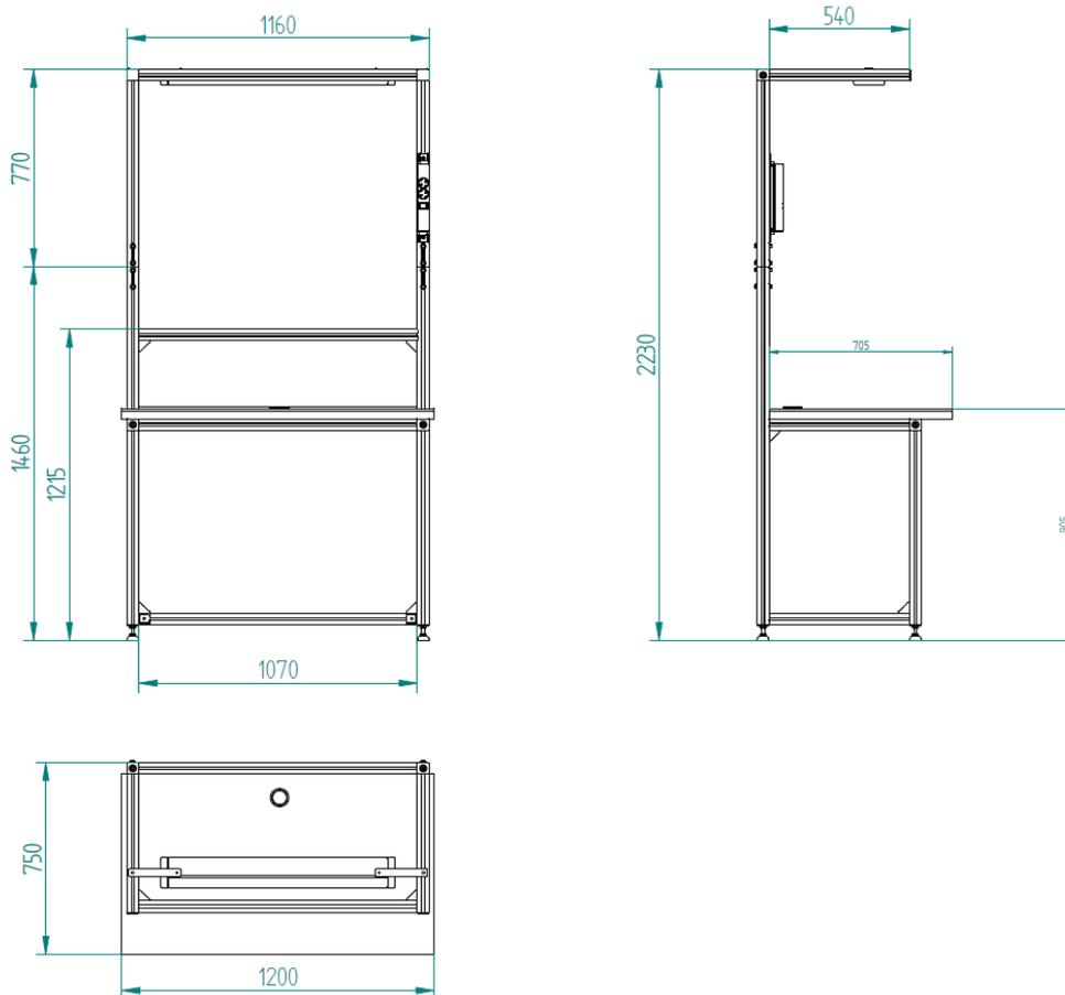
Picture: Dimension Working-station HA-1200 without fixing/ mountings
