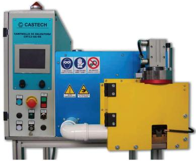
The machine GFA301000 has been developed to connect enamelled wires and cables normally used in the electromechanical industry following the logical of a semiautomatic process combined to easiness of use, flexibility and high productivity so to get the best consistent and repetitive result.
